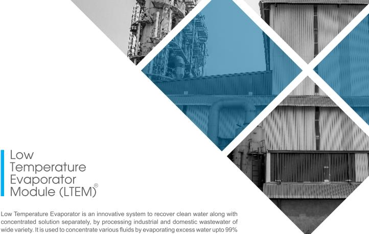
concentrated solution separately, by processing industrial and domestic wastewater of wide variety. It is used to concentrate various fluids by evaporating excess water upto 99% depending on Boiling Point Elevation (BPE) of fluid. All excess water is recovered as clean water or condensate separately along with concentrated fluid.
